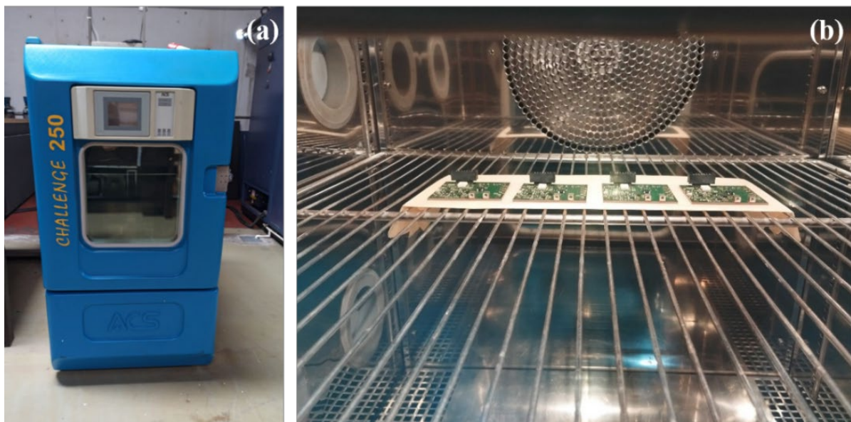
Figure 15 – a) Climatic chamber available at TEKNE , and b) SCs situated within the climatic chamber.
